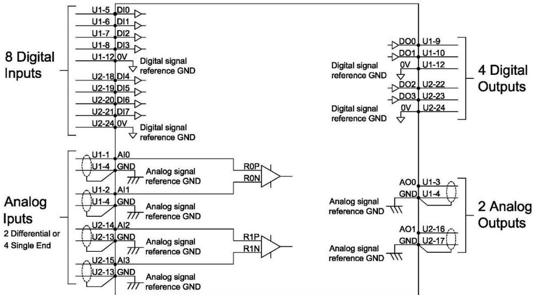
**NOTE:** All analog signal reference GND are the same, and all digital signal reference GND are the same.
