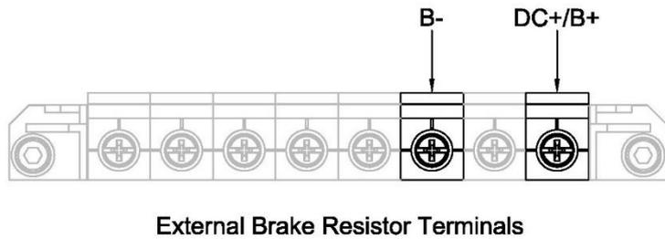
**Step3: Insert Wires into Corresponding Terminals**
