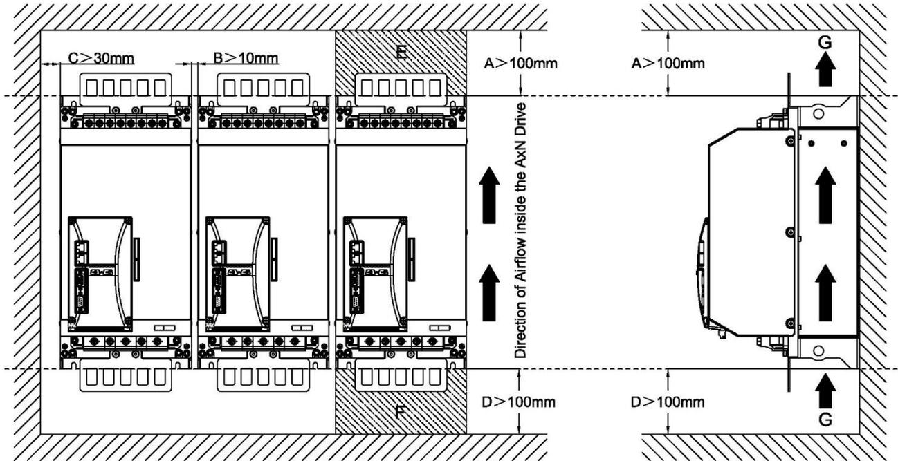
Installation Spacing of AxN Size4 Series Drive
