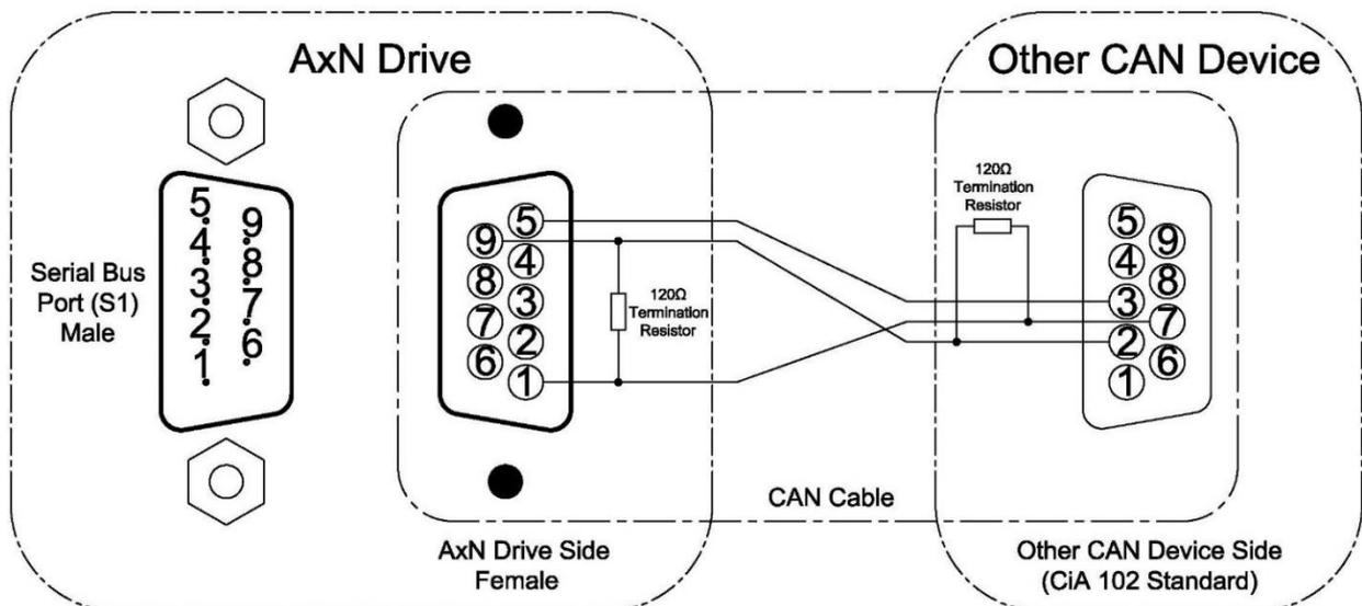
**Note:** Only the first and the last CAN node device should use a 120Ω terminal resistor.
