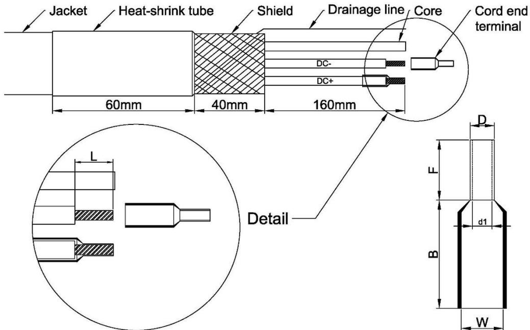
**Step 7: Connect PE wire with Shield**
