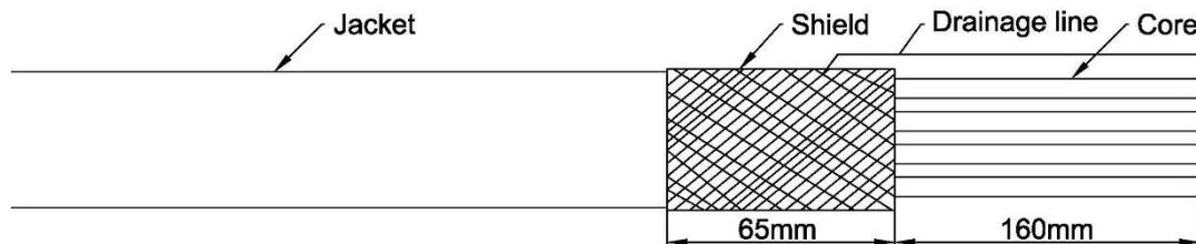
**Step 5: Fix the Grounding Shield**
