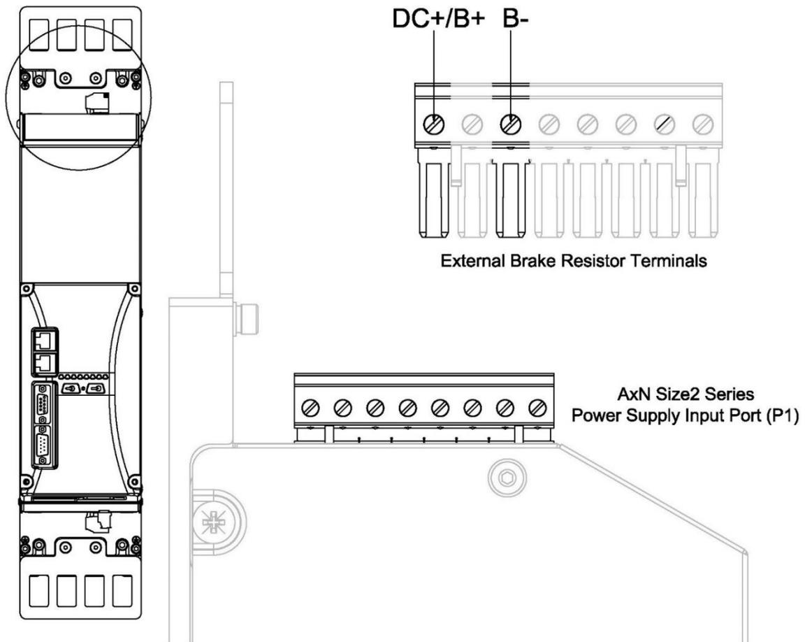
**Step3: Insert Wires into Corresponding Terminals**
