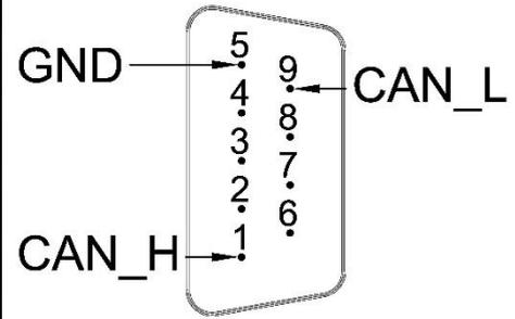
**Note:** CANopen pin assignment on S1 connector does NOT meet CiA 102 Standard.
