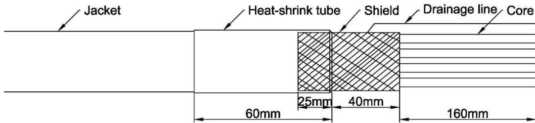
**Step 6: Make the Phase Wires**
